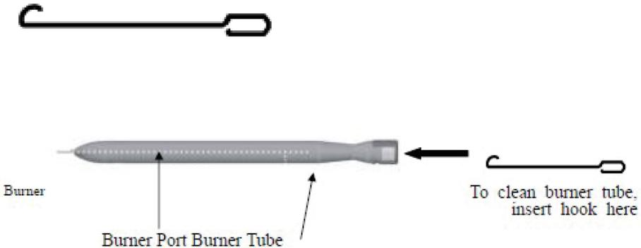
Use a bottle brush with a flexible handle. Run the brush through the burner tube and inside the burner several times, removing any debris.
